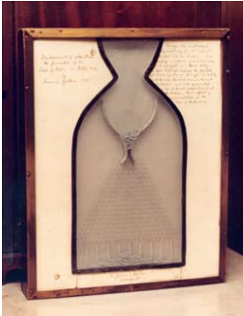
Galton Board on display at the Galton Laboratory, University College London. "Instrument to illustrate the principle of the Law of Error or Dispersion, by Francis Galton FRS." Courtesy Stephen M. Stigler.
